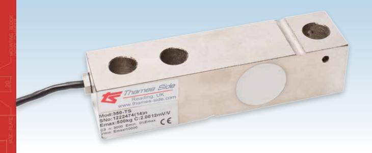
This low cost shear beam load cell is ideal for applications where fully welded, hermetically sealed products are not required. It is manufactured from alloy steel and nickel plated, with the strain gauged pockets protected by a silicone compound for protection to IP66.
