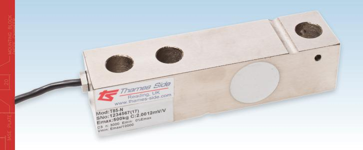
The T85-N low cost shear beam load cell is ideal for applications where a fully welded, hermetically sealed, stainless steel load cell is not required. It is manufactured from alloy steel and nickel plated, with the strain gauged pockets protected by a silicone compound giving protection to IP66.
