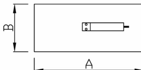
Figure 3. Typical single point installation under a weighing platform
