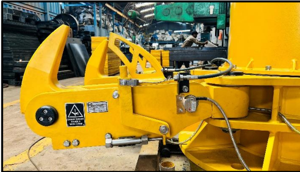
Fig. 1 – QRMH system with integrated ATEX-certified Load Pin
