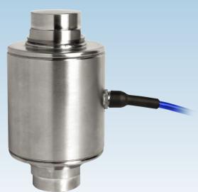
This stainless steel self-centering rocker column load cell is fully welded and hermetically sealed, with protection to IP68 and IP69K. It's an ideal solution for weighbridges (truck scales) thanks to its approval to OIML C4 (4000 divisions) and integral lightning surge arrestors. As well as being extremely tough, the cable's halogen-free Polyurethane sheath has high resistance to rats, chemical attack, cuts, ultraviolet light and temperature changes.
