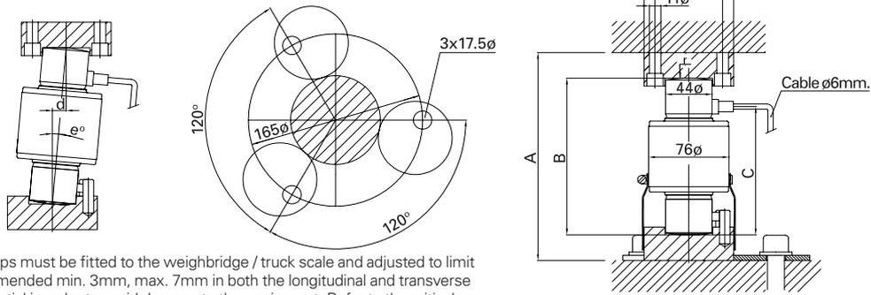
Important: Bumper stops must be fitted to the weighbridge / truck scale and adjusted to limit movement to a recommended min. 3mm, max. 7mm in both the longitudinal and transverse directions. This is essential in order to avoid damage to the equipment. Refer to the critical dimensions d and e below (\*\*).
